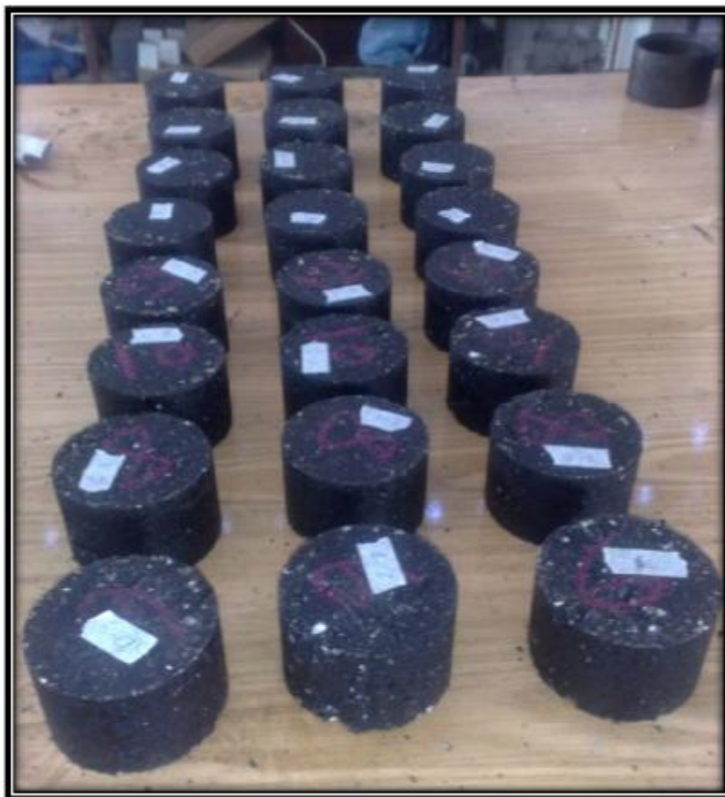
Figure (3.16): WPB modified Marshal Specimens
