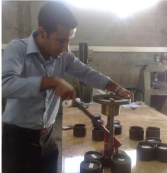
Figure (F.9): Removing Marshal samples molds after compaction
