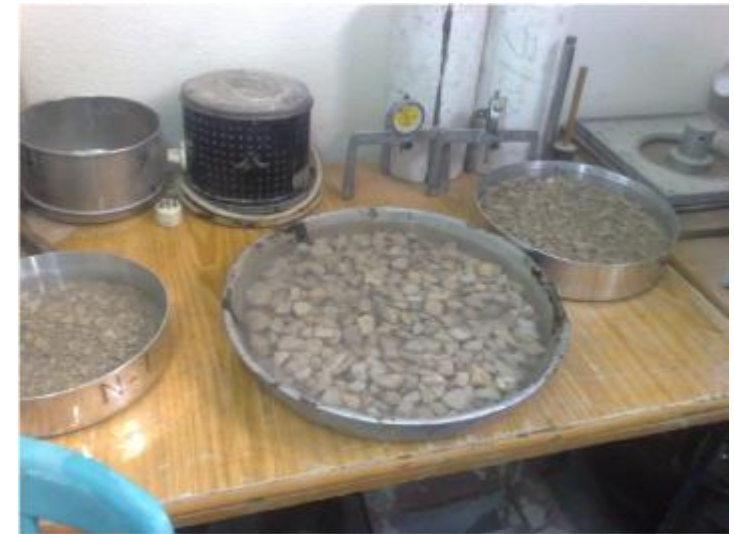
Figure (F.4): Aggregates preparing for specific gravity and water absorption 1
