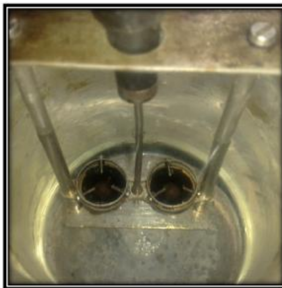
Figure (3.5): Softening point test for bitumen samples
