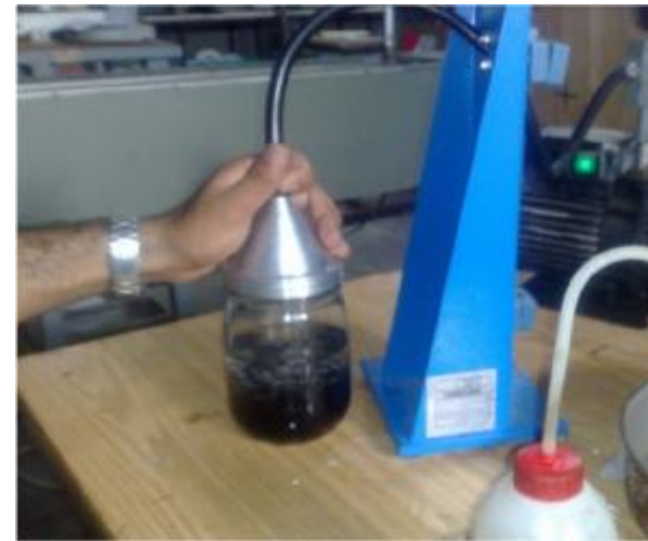
Figure (F.12): Measuring the theoretical density of asphalt mix using Pycnometer
