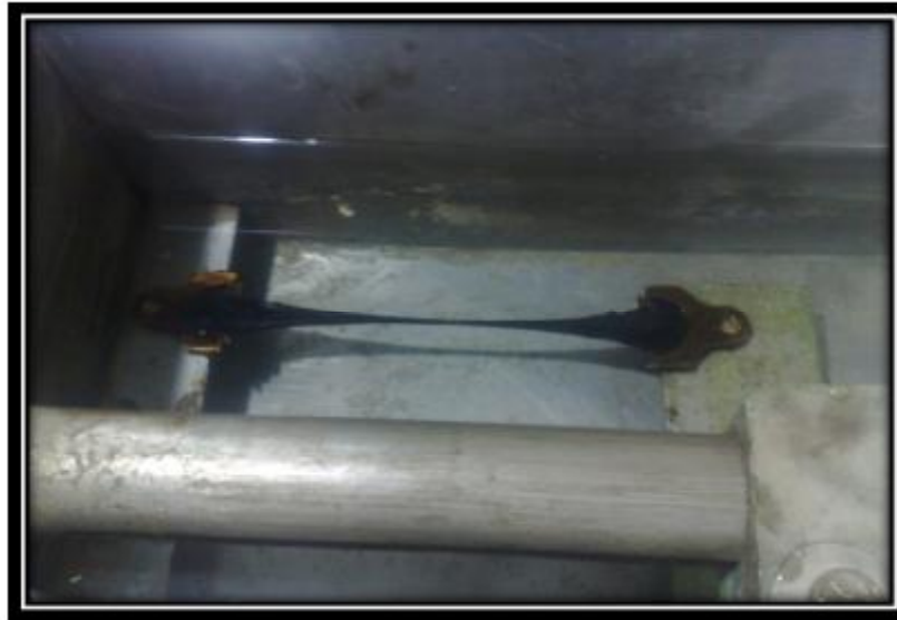
Figure (3.4): Ductility test for a bitumen sample
