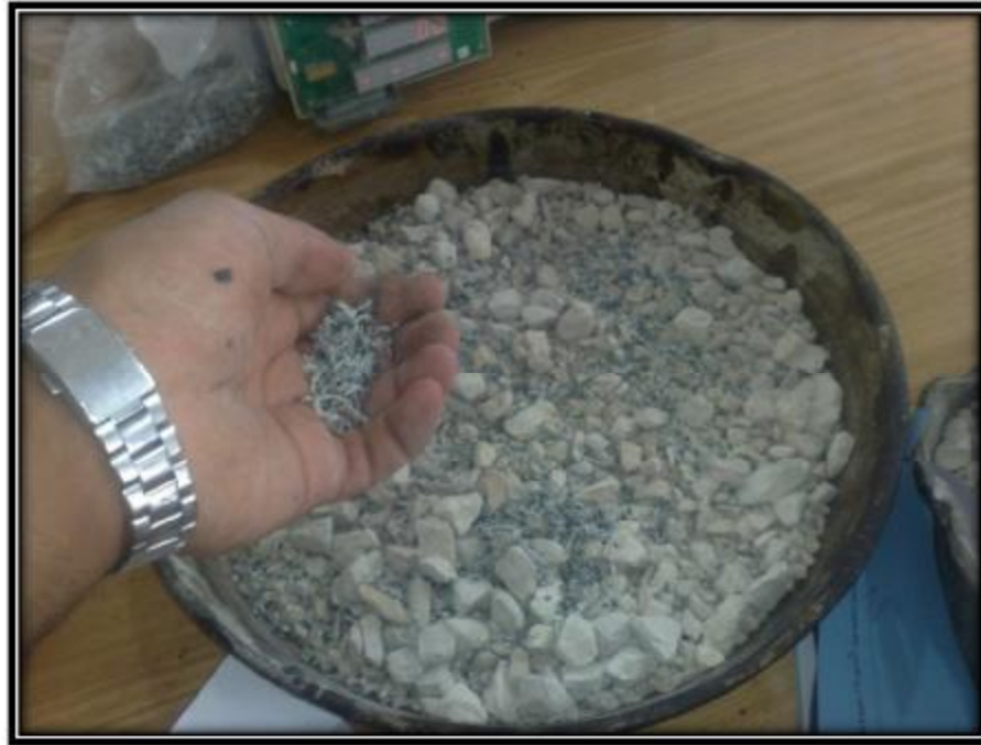
Figure (3.15): Adding WPB to aggregates before heating
