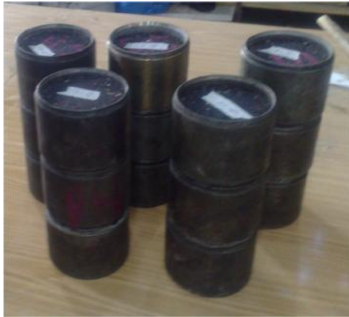
Figure (F.5): Job mix Marshal Samples
