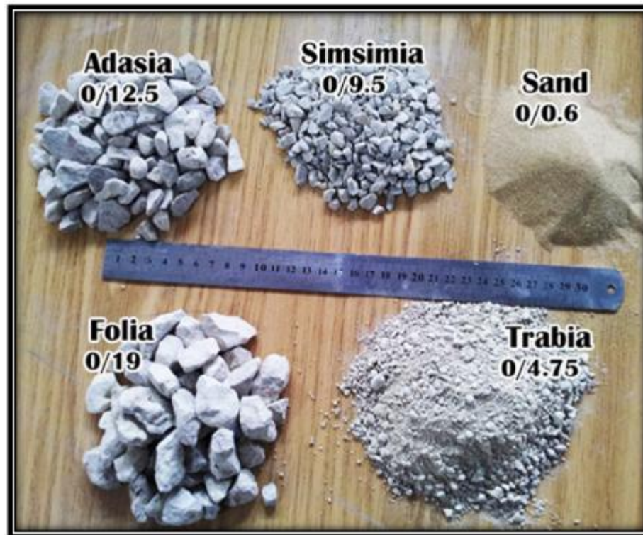
Figure (3.7): Used aggregates types
