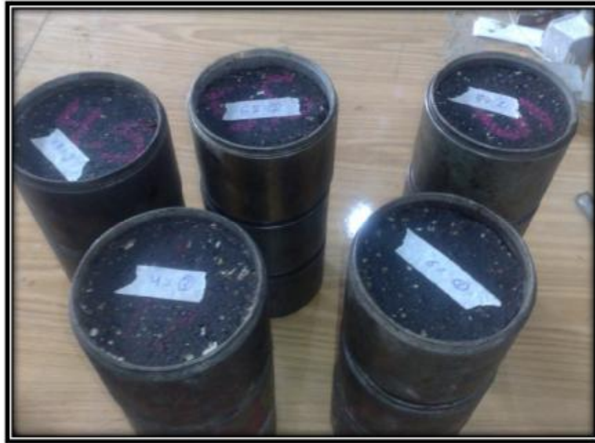
Figure (3.14): Marshall specimens for different bitumen percentages
