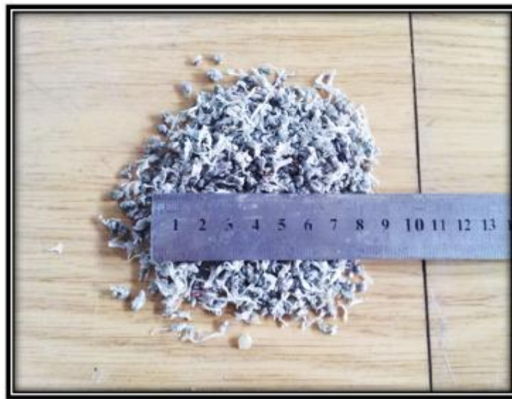
Figure (3.6): Used grinded waste plastic
