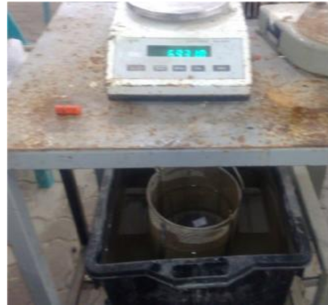
Figure (F.6): Marshal Samples weighing in water
